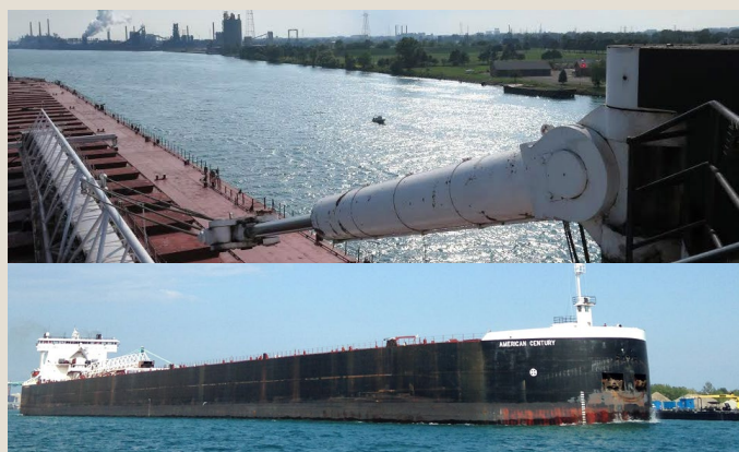
Figure 19. Measuring water velocity as a 1,000 foot freighter travels the Detroit River. View from freighter and research boat. Credit: UM Water Center and USGS.
