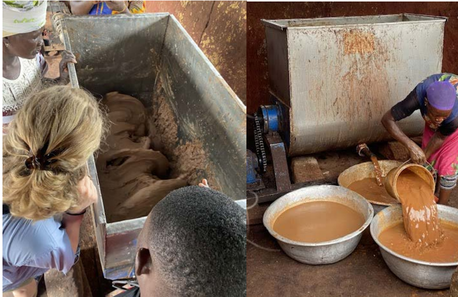
Image 2. Left panel: the inside of a mechanical kneading machine, which separates the solid shea oils from the liquid and cake material. This machine replaced a grueling hand kneading process. Right panel: a woman managing the waste slurry (a mix of shea liquid and cake material) as it is released from the bottom of the mechanical kneader.
