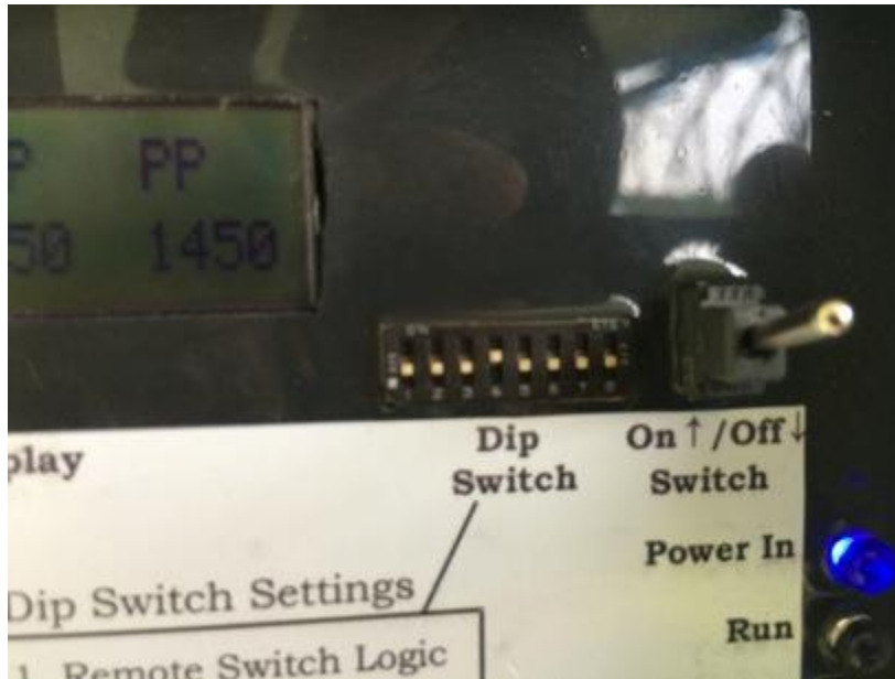
Figure 4. Dipswitch position after installation of system
