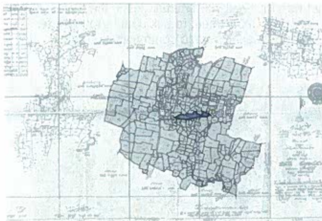
Map 1: Chandaram Village Map Digitized with survey numbers, farmer survey plots, and boundary information. Adilabad, Telangana
