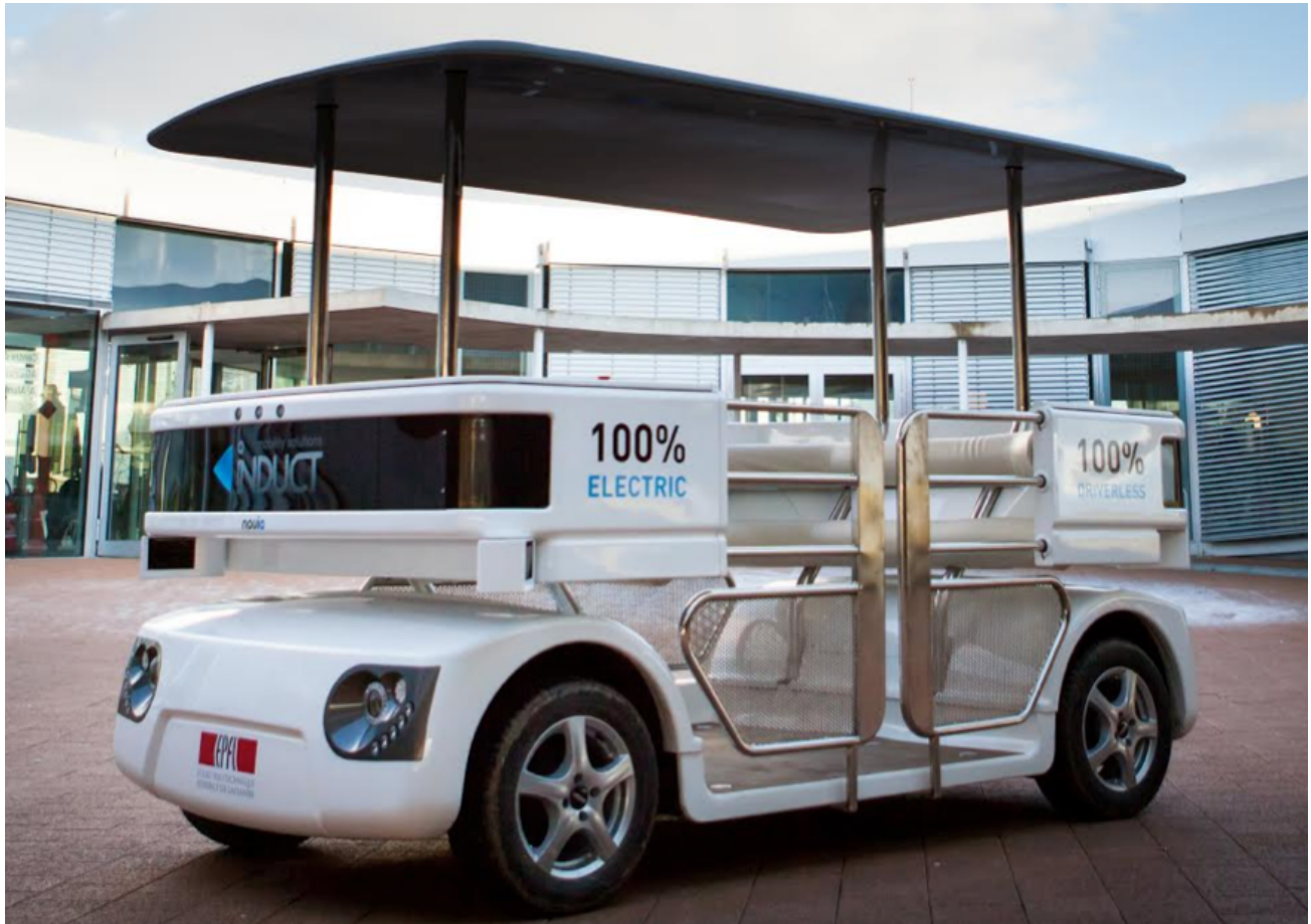
Figure 23. Navia Induct Automated Shuttle, Multiple Passenger Vehicles
