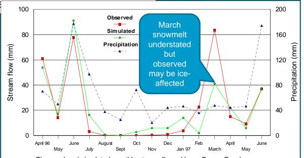
Observed and simulated monthly stream flow - Upper Bower Creek. 1996-97 validation period. Precipitation from USGS weather stations is also shown.
