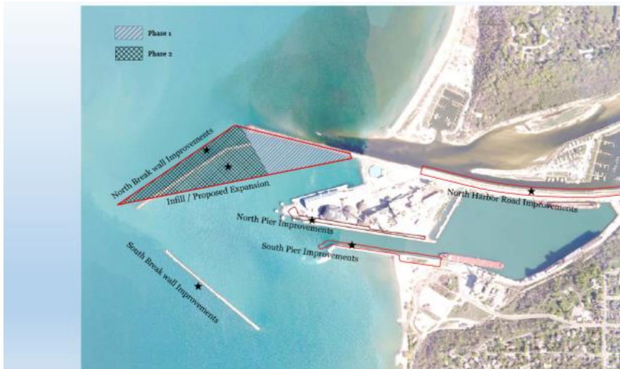
Figure 8: Goderich Harbour Improvements. Source: Goderich Port Management Corporation
