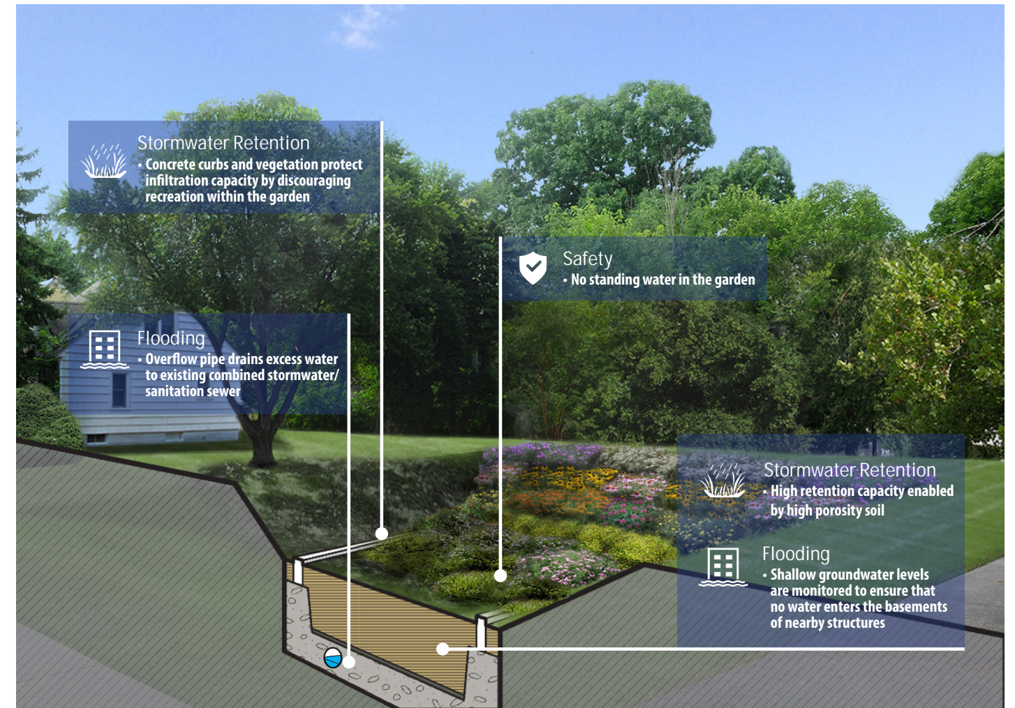
FIGURE 5: Stormwater performance features in bollard garden design. Illustration by QIULING CHEN
