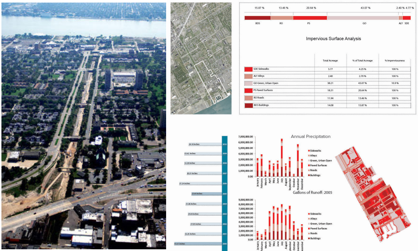
Figure 3.10: Stormwater runoff studies in the Dequindre Cut: land cover delimitation and precipitation data (below)
